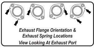
3. Assemble header legs and collector. Install header by slipping onto manifold one header leg at a time. Hook springs onto spring hook on header legs.
