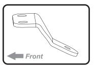
Assemble and secure header bracket to chassis mount bracket as shown. Torque bolt to 23 Nm, 17 ft-lb (2.3 kg-m).
