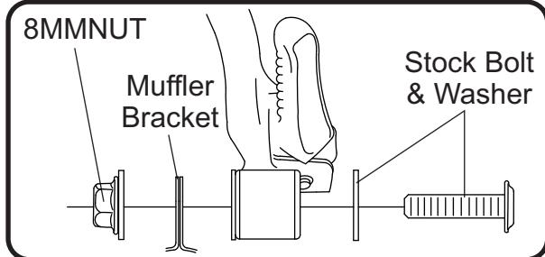
4. Torque muffler mount bolt to factory specification.
