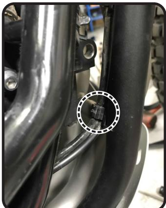
For 2022~ models, remove right front cover to access O2 sensor connector and disconnect. Unclip O2 sensor wire along frame and remove stock O2 sensor.
