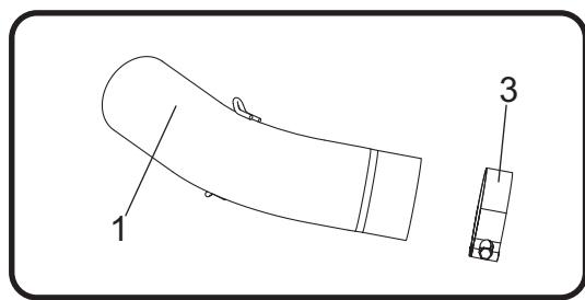
3. Install (No. 1) 14161-435, tailpipe outlet into (No. 2) muffler, inlet.
