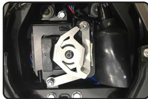
2. Firmly hold servo pulley in place and remove tamper proof torx bolt using the proper torx bit. Install (No. 6) 1464-CKRPLT, servo motor stopper plate on top of the stock pulley as shown above and secure using the stock torx bolt.
