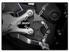
10. Install (No. 5) 13320-RSV-BKT, reservoir bracket using the stock bolt. Secure rear brake reservoir to (No. 5) 13320-RSV-BKT, reservoir bracket using (No. 6) M6X18BHS, bolt (No. 7) 6MMWASHERL, washer and (No. 8) 6MMLN, lock nut. See diagram for proper orientation and order of hardware.
